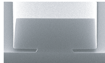
Figure 2. LOL2000 on Si at 200°C/5 min. with 5.0 micron SPR950
